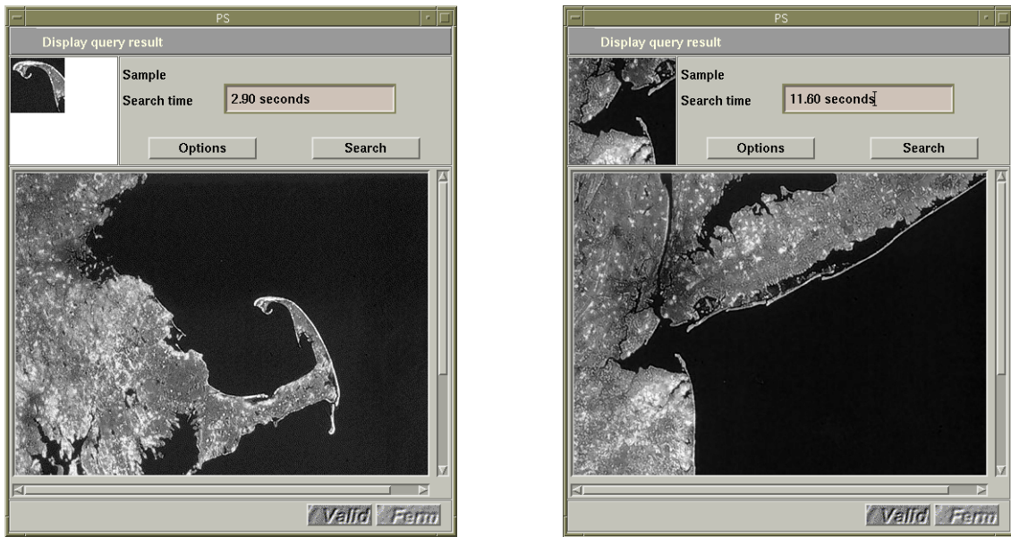
Figure [11]: Results of a query based on a 64x64 pixels pattern (left) and on a 128x128 pixels pattern (right). The database contains 100 images (computed on a SUN SPARCstation 20) (Landsat images).
