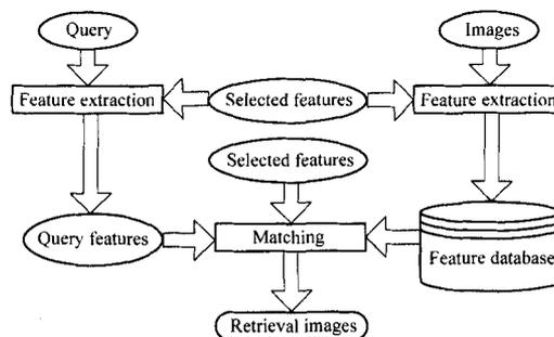
Fig. 1 Diagram for content-based image retrieved system
